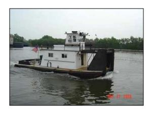
The M/V HERMAN CROWN is a 50' x 18', twin screw, 500 HP towboat of all welded steel construction having a fixed pilothouse and a single level cabin.
